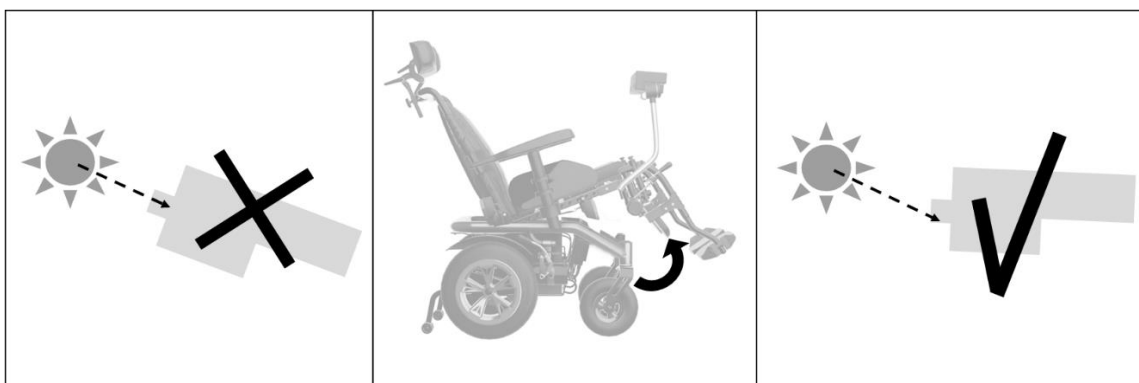
[33] Shows the sun shining into GazeDriver's camera in the normal upright driving position. By tilting the wheelchair, the sun is prevented from shining directly into the camera, with which driving control can again be achieved.
